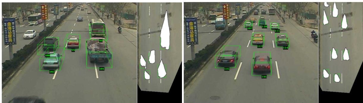
Figure 10: Fusion result of vehicle identification and tracking
