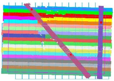
Figure 3. LIDAR strips and control fields (red dots).
