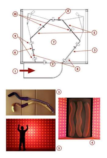
Figures 2 and 3: Design of the space and photographs of the interactive areas. 1: Access ramp. 2: Entrance. 3: Tune fork tactile and auditory wall. 4: Vibrating interactive wall. 5 & 6: Projection screens. 7: Observation wall. 8: Interactive floor. 9: Microphones and speakers scattered throughout the area. 10: Cameras capturing the images.
