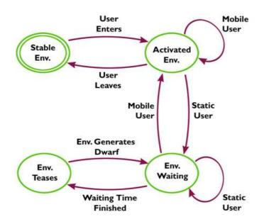
Figure 5: exampe of Fullaraca, one of the automata developed that describes the states that the model can have as a function of user interaction.
