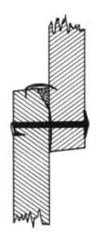
the planks of the clinker-built sides of the Bremen cog are kept together by iron nails, the points of which are bent again into the inside of the planks and the caulking is covered by narrow laths kept in position by flat iron caulking clamps, which in Hanseatic times were known as «sintel». Several of these constructional details prove that the Bremen wreck, built in ca 1170 (fig 6), was the fragment of a cog.
