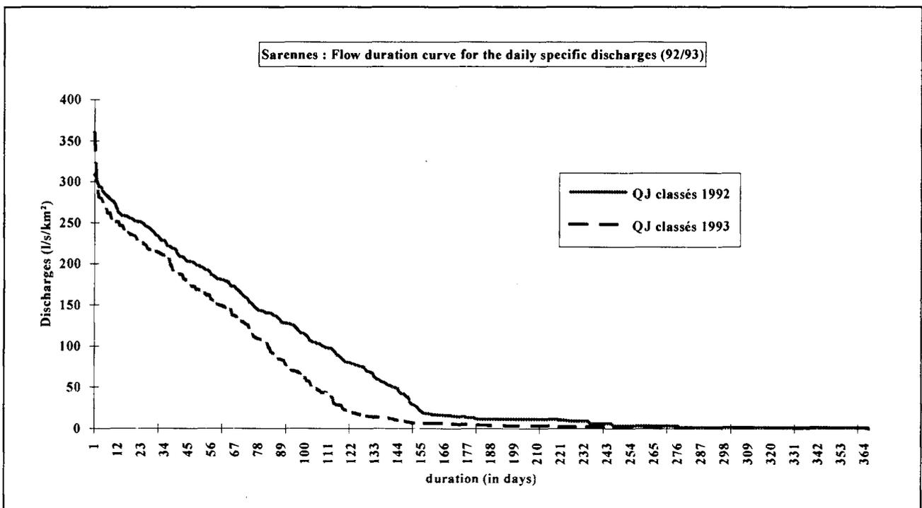
Figure 8. Flow duration curve for the two years 1992 and 1993 (from daily specific discharges)
