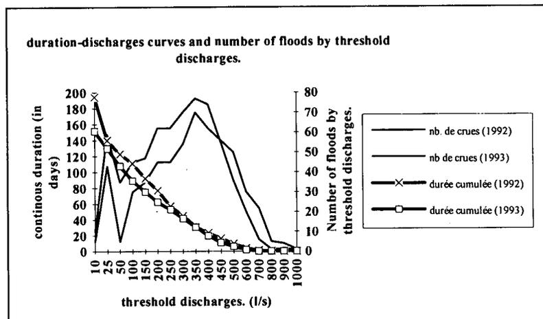
Figure 16. Discharges-Durations curves and number of floods by threshold discharges.
